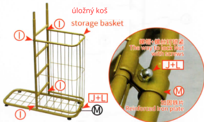
The installation of Iron plate:
